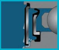
Once the stream is directed away from the wheel, the deflected shield returns to its original position, allowing any residual fluid that entered the area between the shield and seal to drain out or be spun out by centrifugal force.
